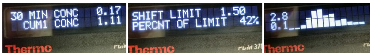
Figure 2.3. Information displayed on a PDM3700. The first PDM screen shows 30-minute and cumulative concentration (left), the second screen shows shift limit and percentage of limit (center), and the third screen shows a bar chart of 30-minute averages (right).
