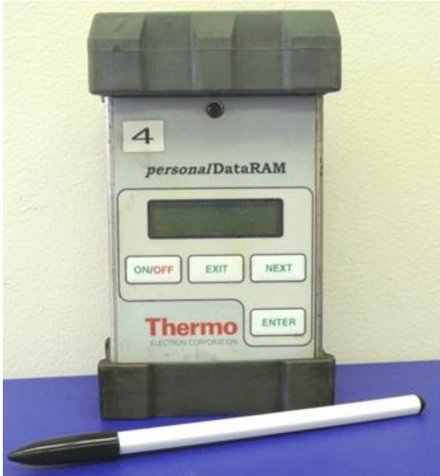
Figure 2.4. pDR 1000AN sampler (left) and pDR operated with gravimetric samplers in an underground coal mine (right).
