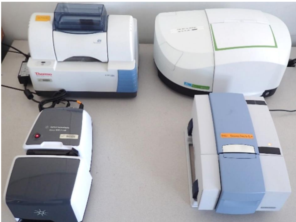
Figure 2.6. Portable FTIR units used in NIOSH testing: Thermo Fisher (top left), Perkin Elmer (top right), Bruker Optics (bottom right), and Agilent manufacturers (bottom left).
