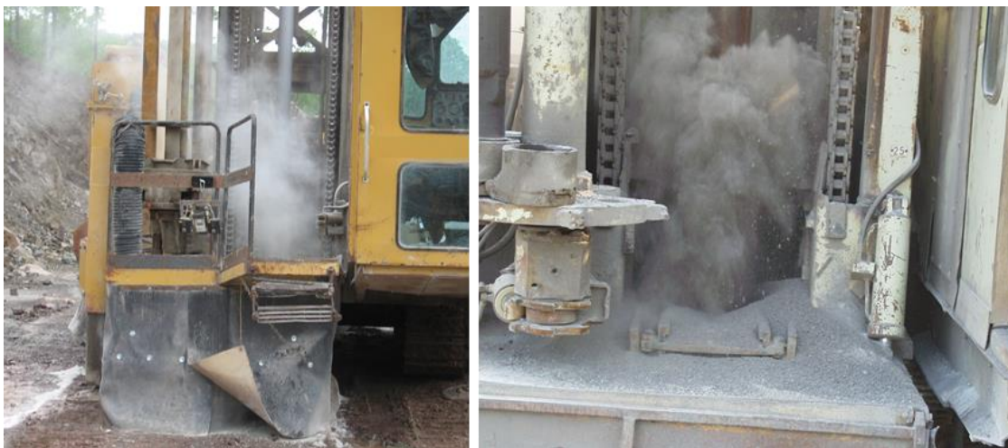
Figure 5.7. Dust leakage through drill stem bushing on two different drills.
