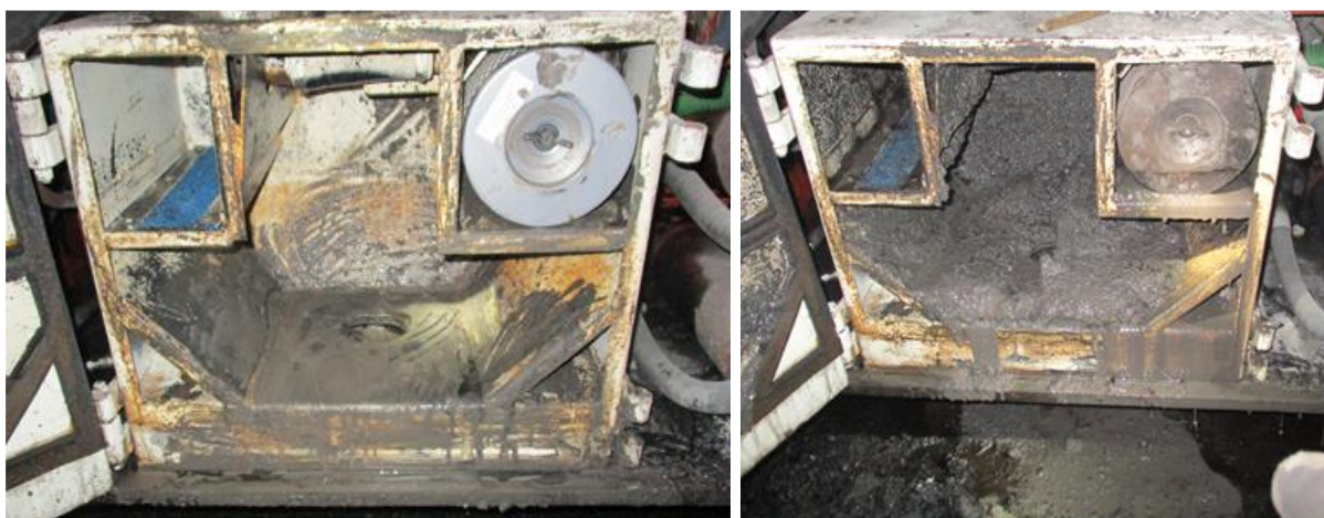
Figure 4.26. Wet collector box on roof bolter (left) and wetted material in collector box (right).
