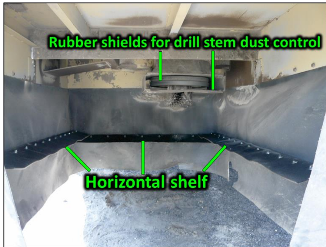
Figure 5.5. Air-blocking shelf installed on drill shroud (left) and laboratory test configuration showing leakage through gaps in the drill shroud and blocking shelf (right).
