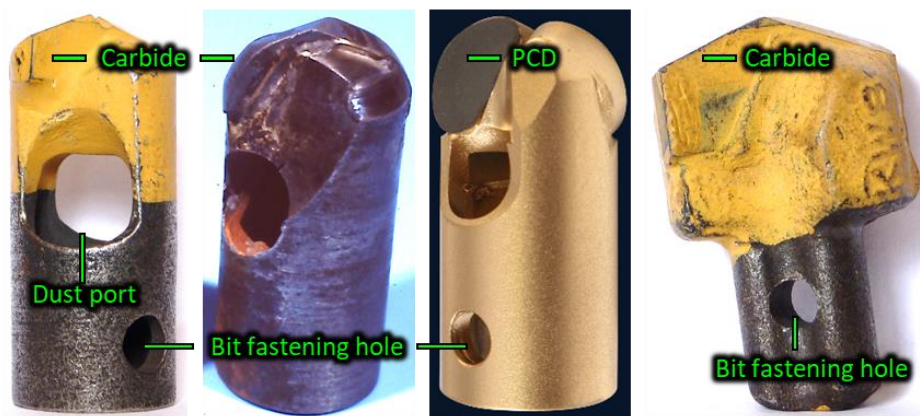
Figure 4.17. New (left) and worn (left center) tungsten carbide dust hog style bits, polycrystalline diamond (PCD) dust hog bit (right center), and shank-style bit (right).
