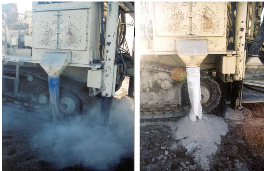
Figure 5.9. Dust at collector dump before (left) and after shroud installation (right).
