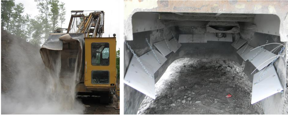
Figure 5.6. Dust released when material drops off of air-blocking shelf (left) and modified design with short, overlapping sections supported by chains to maintain the 45-degree angle (right).
