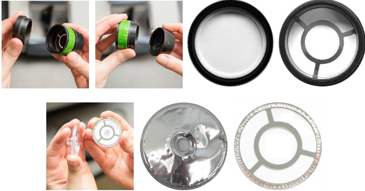
Figure 2. Examples of suitable sample cassettes (which allow the filter media to remain secured in the cassette or capsule) for field-based analysis. The holder or cassette containing the filter media with the sample should be open on both sides, which can be accomplished by removing the top and bottom cassette pieces of the four-piece cassette (top) or removing the capsule from the dust sampling cassette (bottom). From one side the dust material on the filter (or a portion of the filter, in the case of dust sampling capsule) should be visible, and from the other side the underside of the filter media should be exposed and the support ring should be visible.
