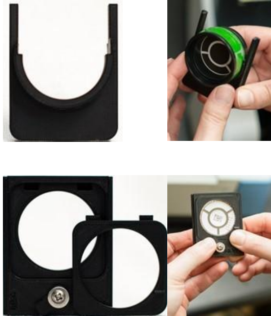
Figure 3. Inserting the sample into the cradle or holder. NIOSH has designed a cradle (top left) to accommodate the four-piece cassette (top right) and a filter holder (bottom left) to accommodate the dust sampling capsule (bottom right). The four-piece cassette should be inserted firmly into the cradle so that the sample is not tilted forward or backward in the cradle. The dust sampling capsule should be centered in the holder and secured so that the sample remains stationary when the holder is held vertically. Files of 3D models of the cradle, the filter holder, and instrument brackets (for each of the four portable instruments, for 3D printing or traditional machining) that fit either option are freely available at https://3dprint.nih.gov/discover/3dpx-013209 .
