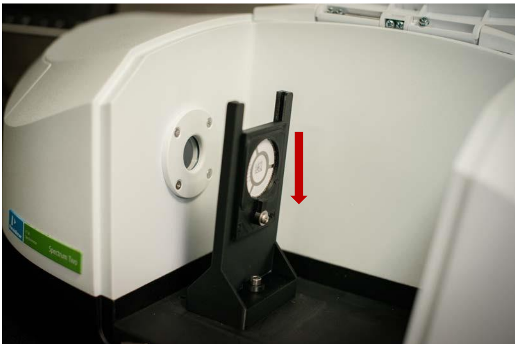
Figure 4. Placing the cradle or holder in the transmission compartment of the FTIR instrument. The cradle (top) or the filter holder (bottom) should be inserted fully into the sample bracket in the instrument so that the bottom of the cradle or filter holder is tightly in contact with the sample bracket.
