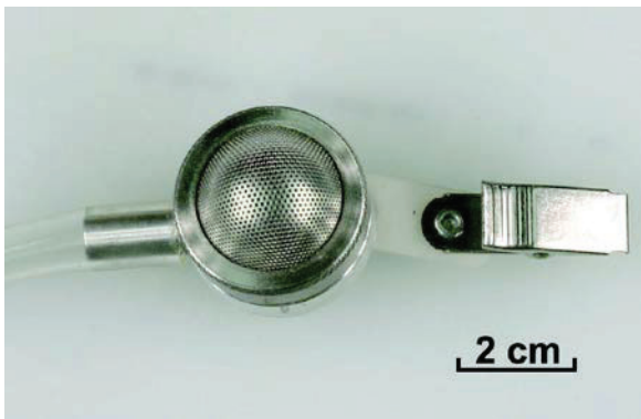
Figure 2D. Button sampler. So-named because the inlet, a hemispherical screen with ~380 \mu\text{m} diameter holes, resembles a large button. It was developed as an inhalable sampler with reduced wind direction response and improved filter deposit uniformity. The sampler uses metal construction and operates at 4 L/min.
