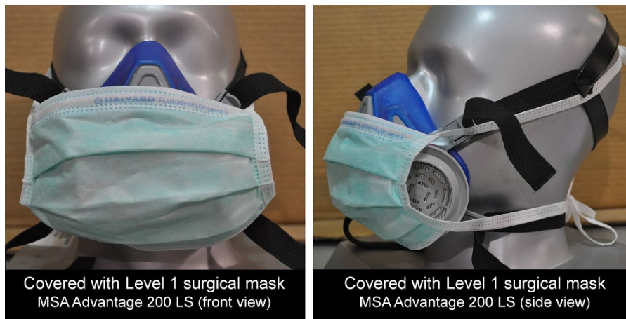
Figure 4. MSA Advantage 200 LS covered with Level 1 surgical mask donned on a headform. The MSA Advantage 200 LS exhalation valve is positioned on the front of the facepiece and frontward facing. The center of the surgical mask is aligned over the exhalation valve and results in partial coverage of the filters, but this partial coverage was assumed not to affect inhalation resistance or airflow direction.
