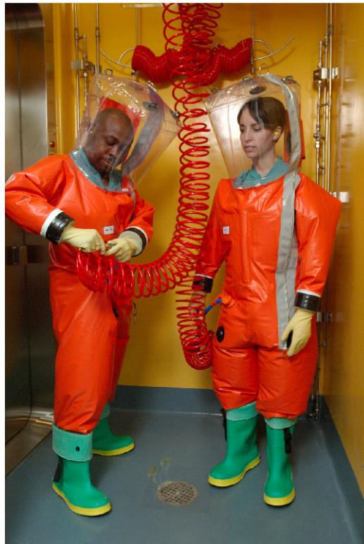
Figure 13.2 A protective suit like this one is an additional precaution for those who work in BSL-4 laboratories. This suit has its own air supply and maintains a positive pressure relative to the outside, so that if a leak occurs, air will flow out of the suit, not into it from the laboratory. (Credit: James Gathany, CDC, public domain)
