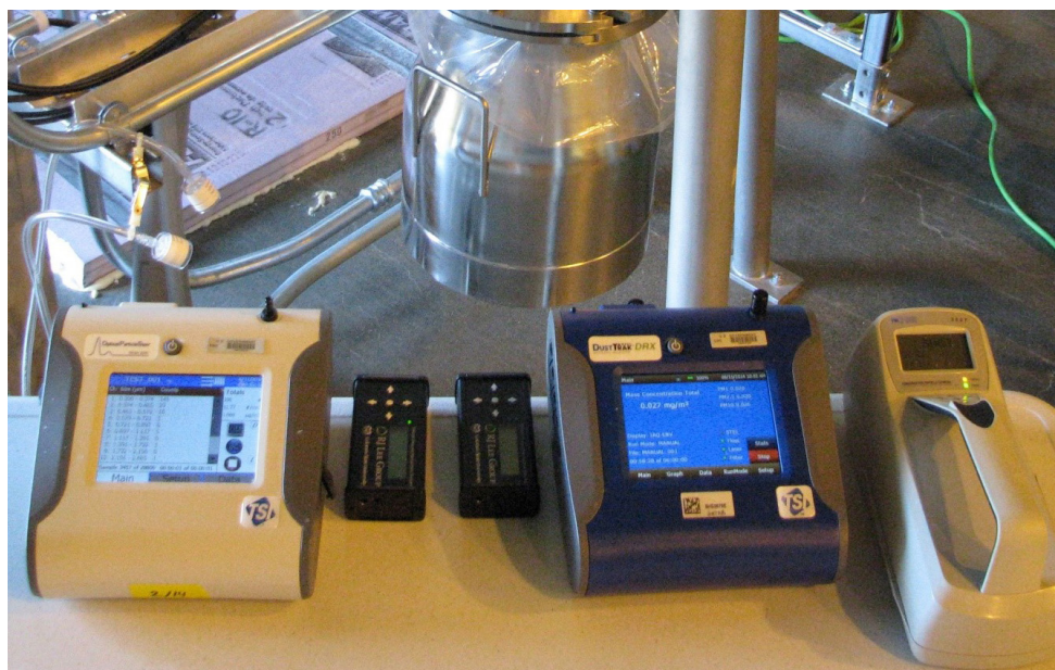
Figure 5. Area sampling shown in the figure includes three real-time data logging particle counters (one condensation particle counter and two optical particle counters), two 25-mm open-face filter cassettes, and two thermophoretic samplers (Photo by NIOSH).
