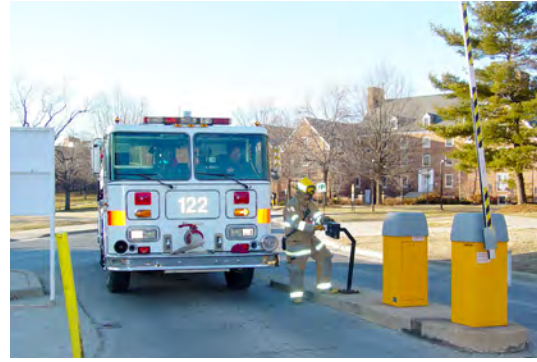
Figure 3.14. An entrance to a private fire lane. The delays caused by electronic gates can be minimized by providing the fire service with access cards or remote access controls.
