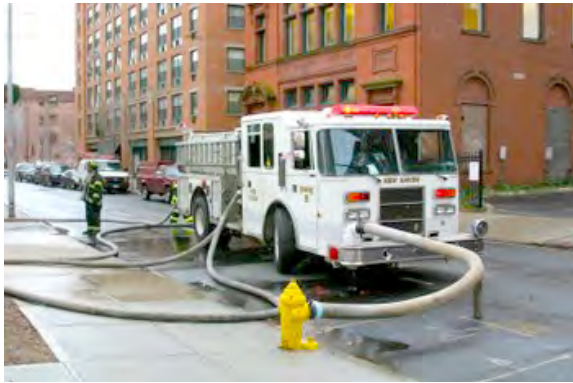
Figure 4.1. A pumper supplying water from a fire hydrant to a fire scene.
