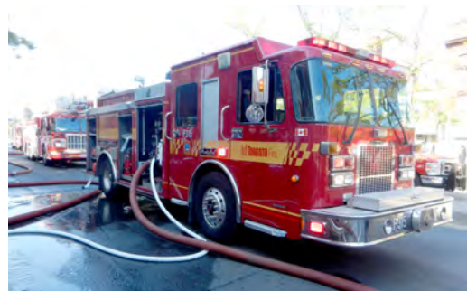
Figure 2.4. A pumper operating at an incident. The red hose is supplying water from a fire hydrant to the pumper. The white hose is a fire attack line.
