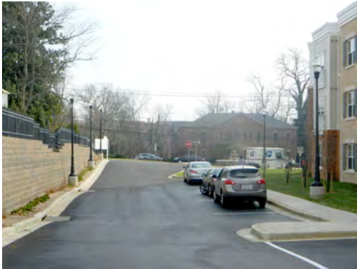
Figure 3.5. The parking spaces on the right do not reduce the width of this fire lane.
