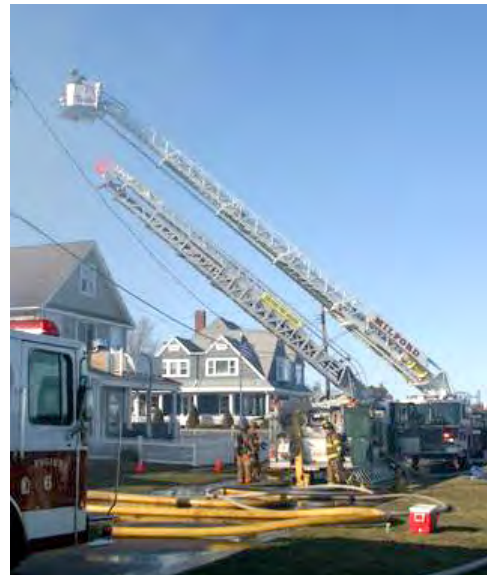
Figure 2.6. Two types of fire service aerial apparatus — one with a straight ladder (left) and the other with an elevating platform (right). The latter type of aerial apparatus is often referred to as a “tower”, “tower truck”, or “tower ladder”.
