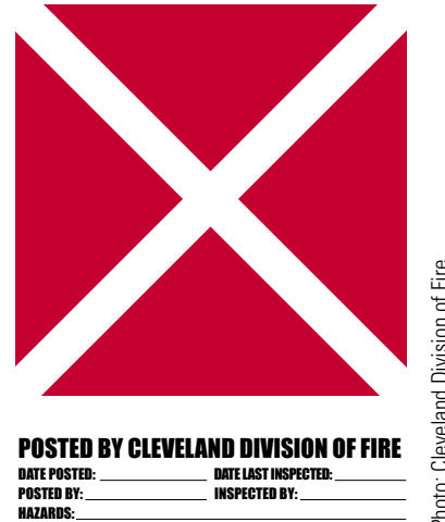
Figure 7.4. A vacancy status sign that warns firefighters that a building is unsafe to enter. Space at the bottom of the sign is for information on specific hazards.
