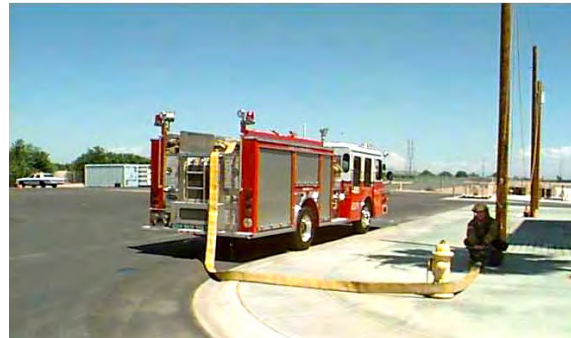
Figure 4.10. A pumper stopped to initiate a straight hose lay from a hydrant.
